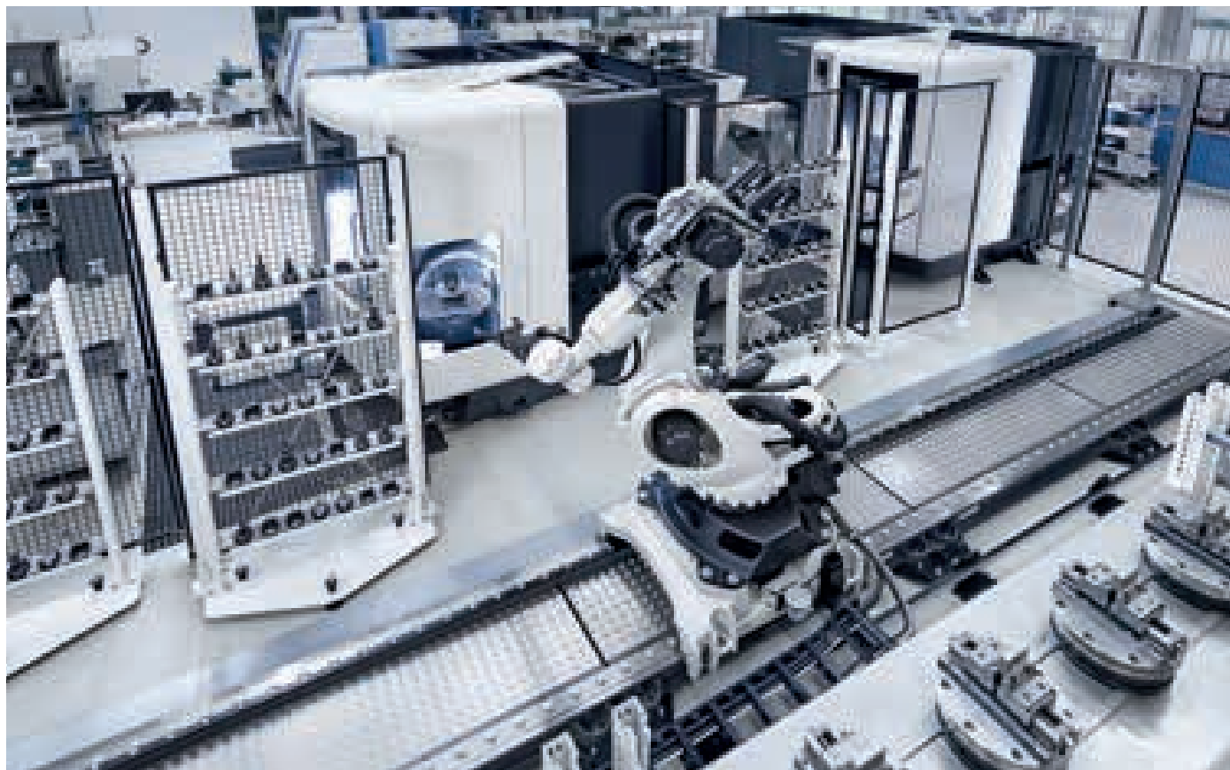
Flexible manufacturing cell with two DMU 60 eVo, one DMU 70 eVo, one robot on the 7th axis and CAD/CAM connection to the process control computer for controlling the machine and tooling requirements as well as order prioritisation.
