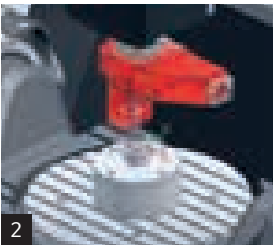
2 3D simulation for collision avoidance, taking into consideration the integrated laser head.
