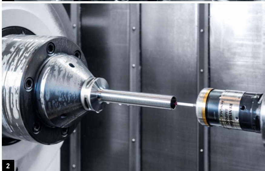
1. Thanks to the large working area of the NTX 3000, Sandvik Coromant Trondheim can easily machine tool bodies with diameters from \varnothing 16 mm to \varnothing 80 mm. 2. Sandvik uses in-process measurement for each workpiece. Post-process measurement outside the machine is thus reduced to occasional spot checks.
