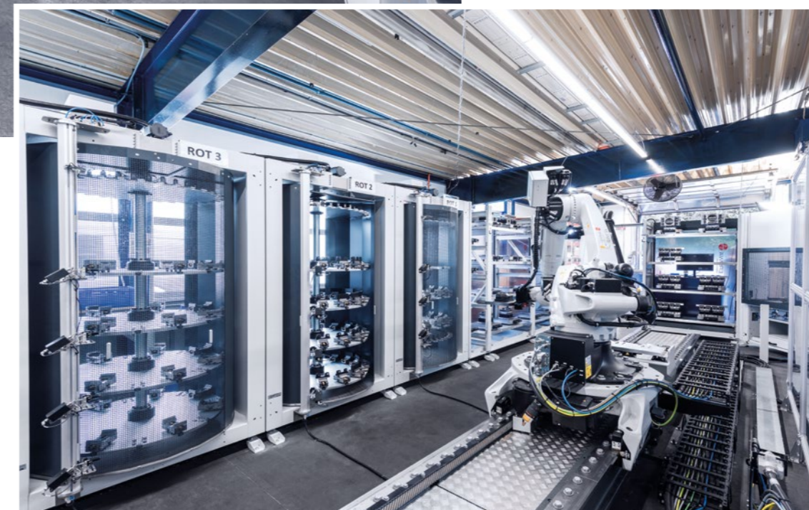
Two of the seven DMU 60 eVo machines are connected via a pallet handling system. This has 40 pallet locations and also has room for 300 fixtures which can be swapped onto the pallets.
