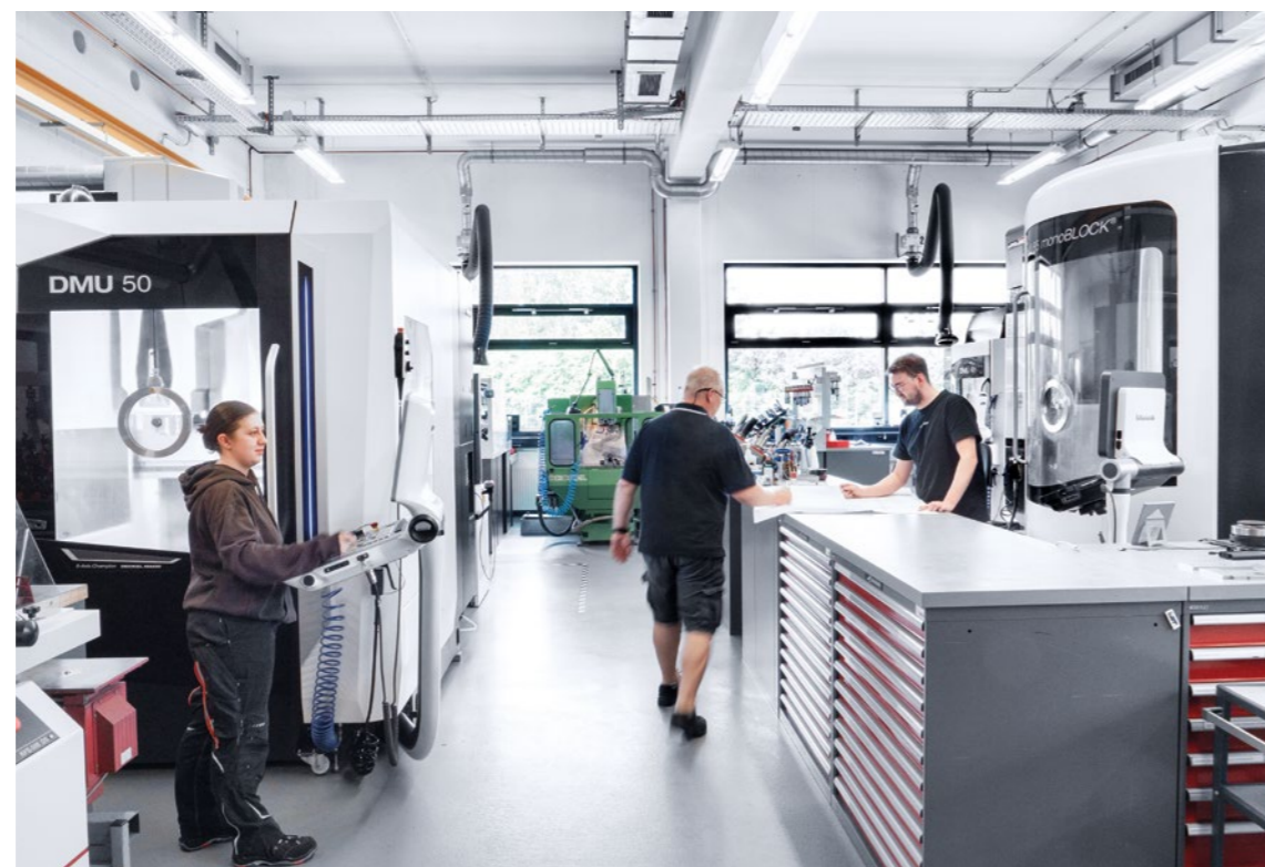
The Max Planck Institute relies on the accuracy of 5-axis machines from DMG MORI for the production of its high-precision optical instruments. A DMU 50 and a DMU 65 monoBLOCK are used here in addition to a DMU 40.
