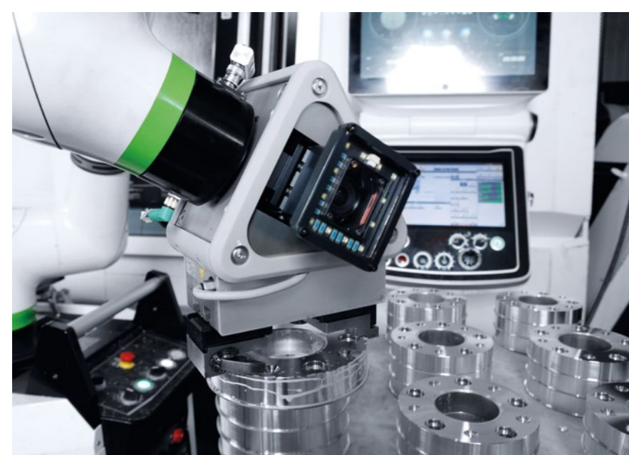
Vision Camera automatically detects the workpiece location and adjusts the arm motion to continue production regardless of misalignments.
