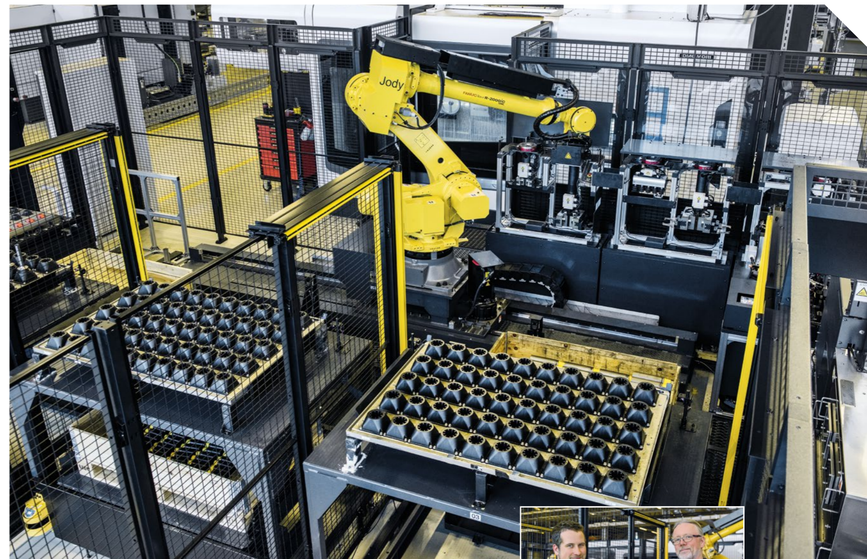
The automated NTX 3000 processes up to 150 components and ensures sufficient production capacity over four unattended shifts.
