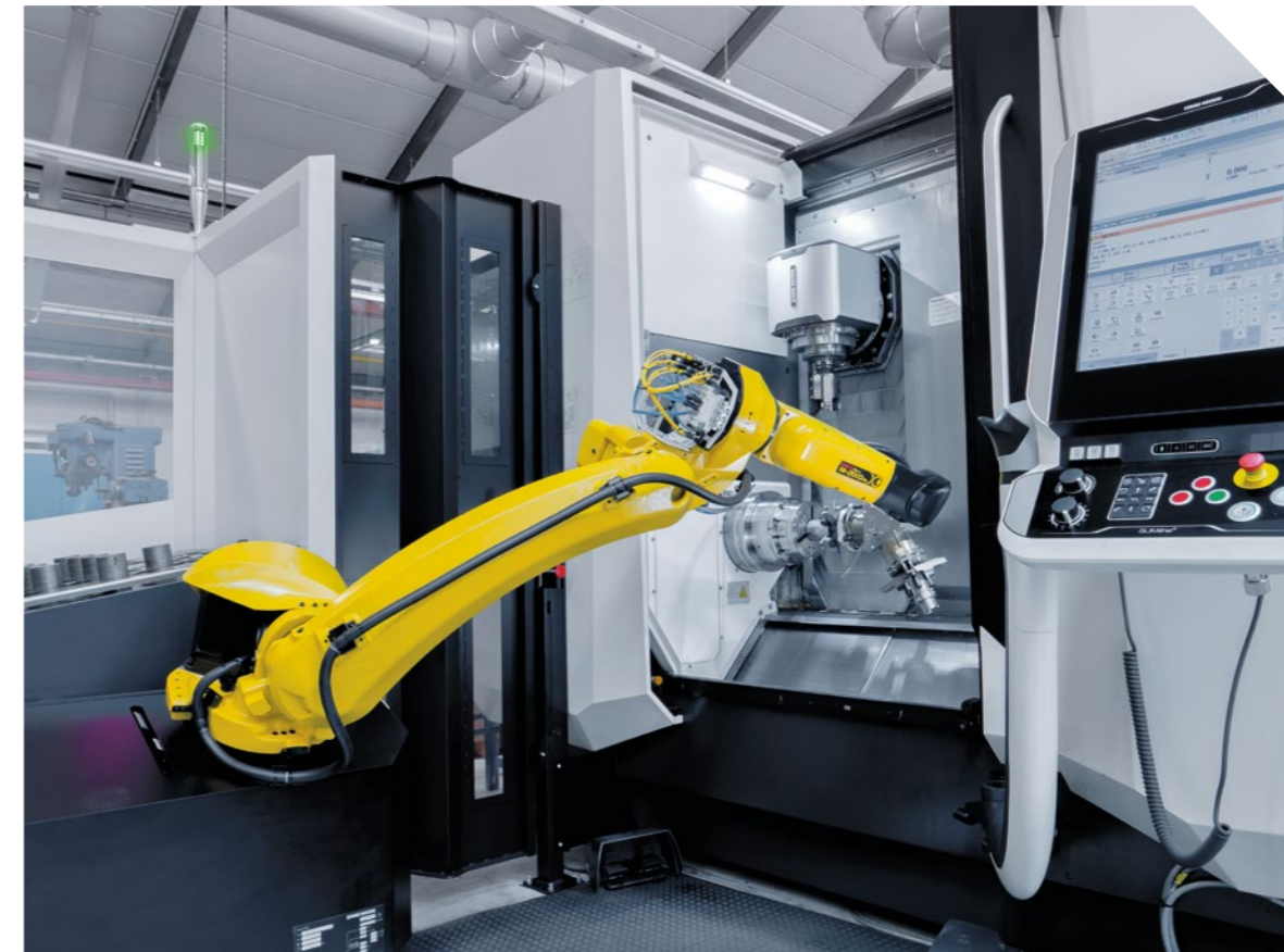
Small batches with short run times are manufactured on the CLX 450 TC during the day. At night and over the weekend, batch sizes of up to 30 parts and more, depending on running times, are produced without operator attendance.
