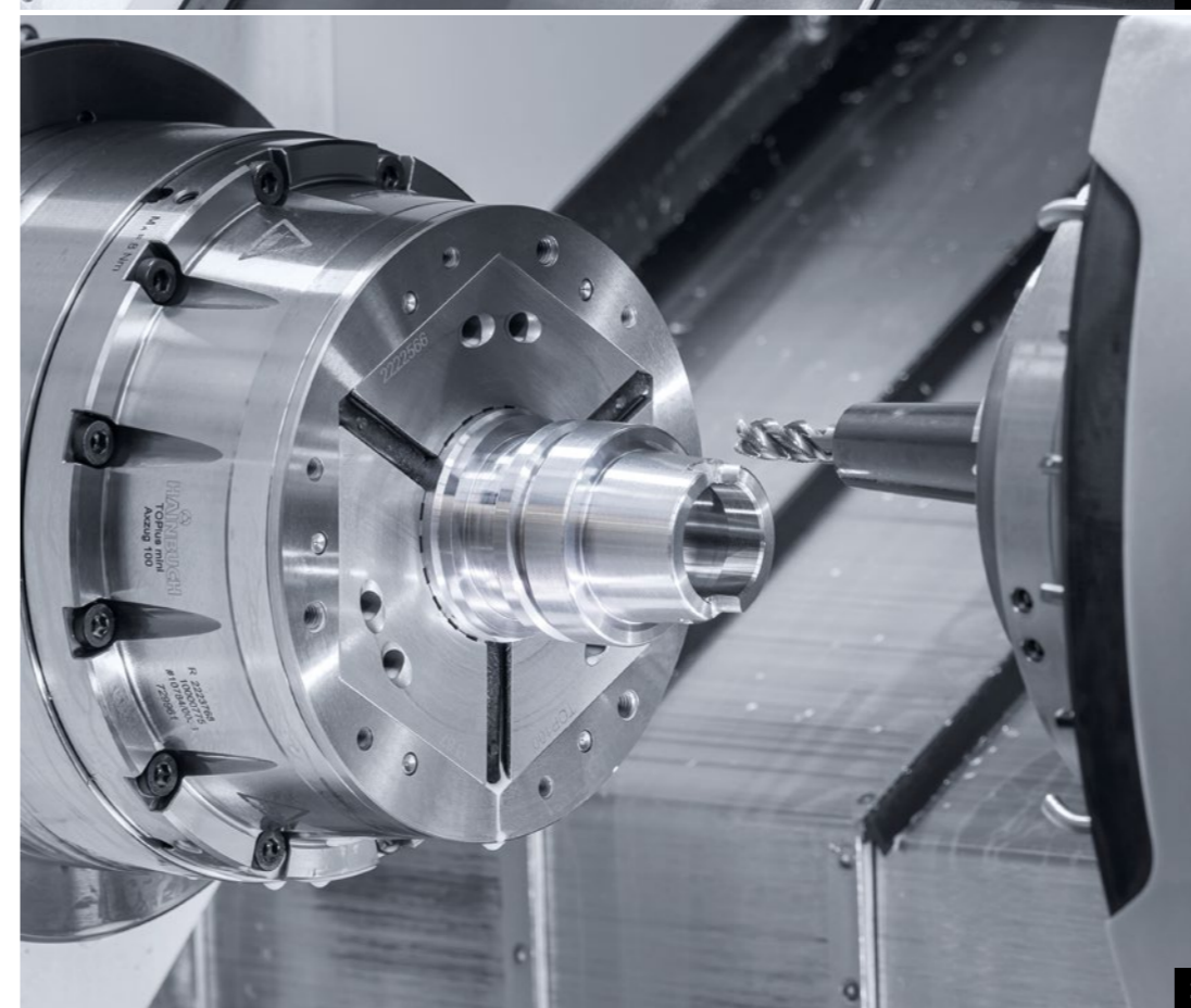
1. The grippers of the Robo2Go can handle the entire component range from \varnothing 25 – 100 mm. 2. Size 32 to 160 HSK tool holders are manufactured on the CLX 450 TC, among other components.
