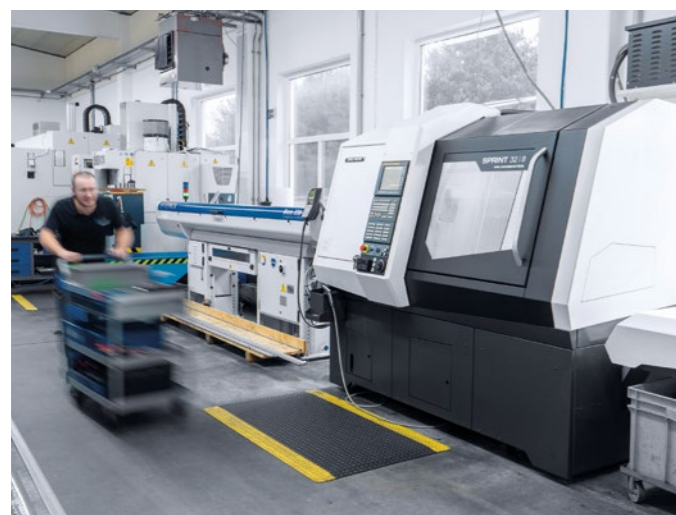
SPRINT 3218: Up to 28 tool locations on 2 independent linear tool carriers enable highly productive production of workpieces with a diameter of up to 32 mm.
