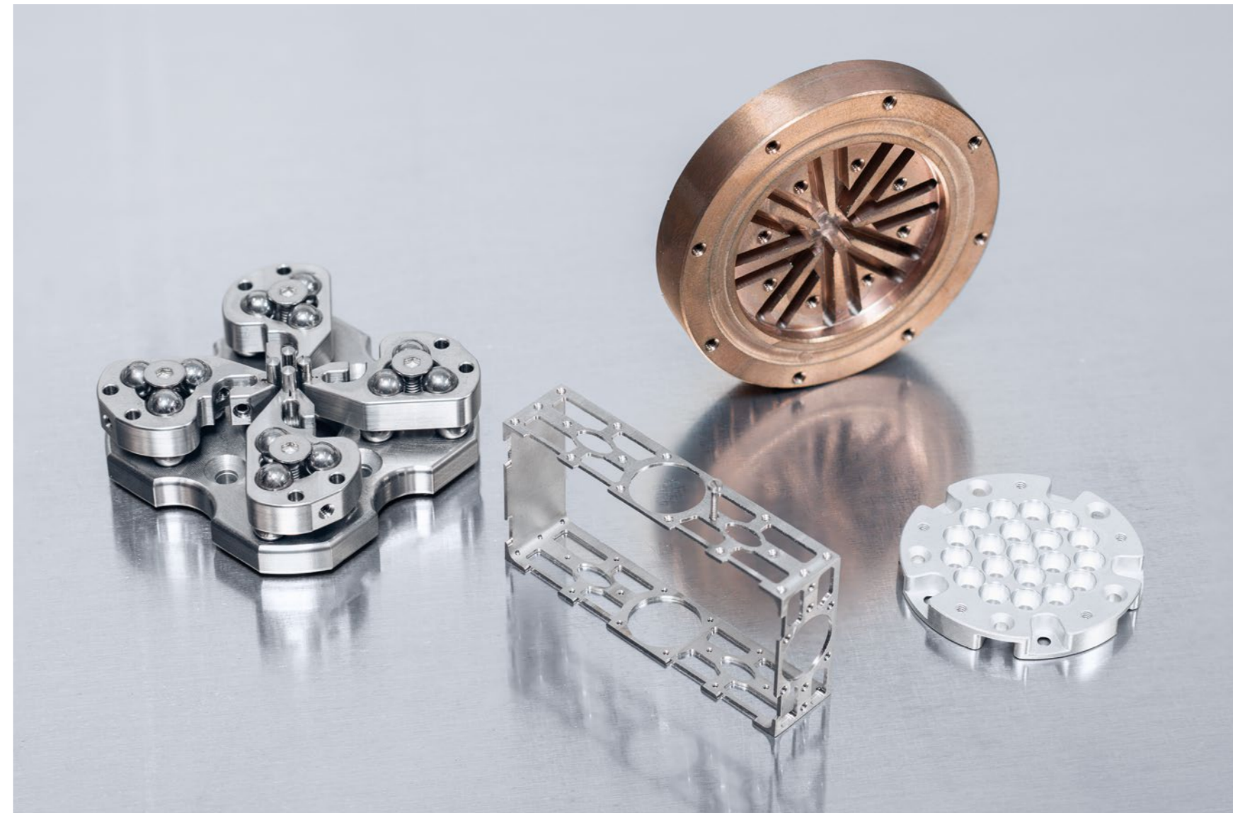
The Max Planck Institute develops and builds high-precision apparatus for its research in the fields of laser development and quantum physics. Such components are produced, in part, on high-precision 5-axis machines in its in-house workshop.
