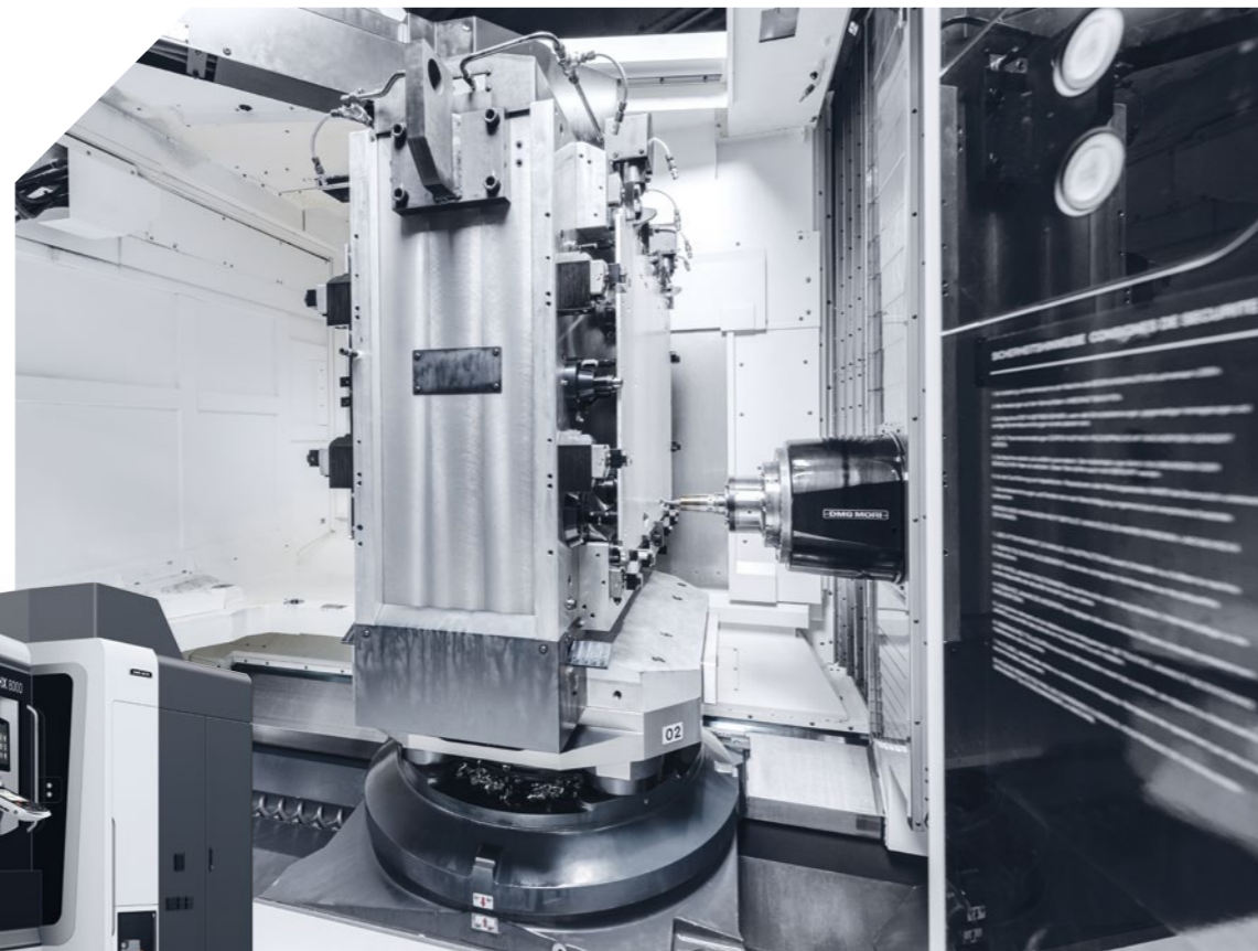
Each NHX 8000 has a pallet changer with one fixture per pallet, each of which is equipped with a panel at both sides. Two floor panels are manufactured in a single machining process.
