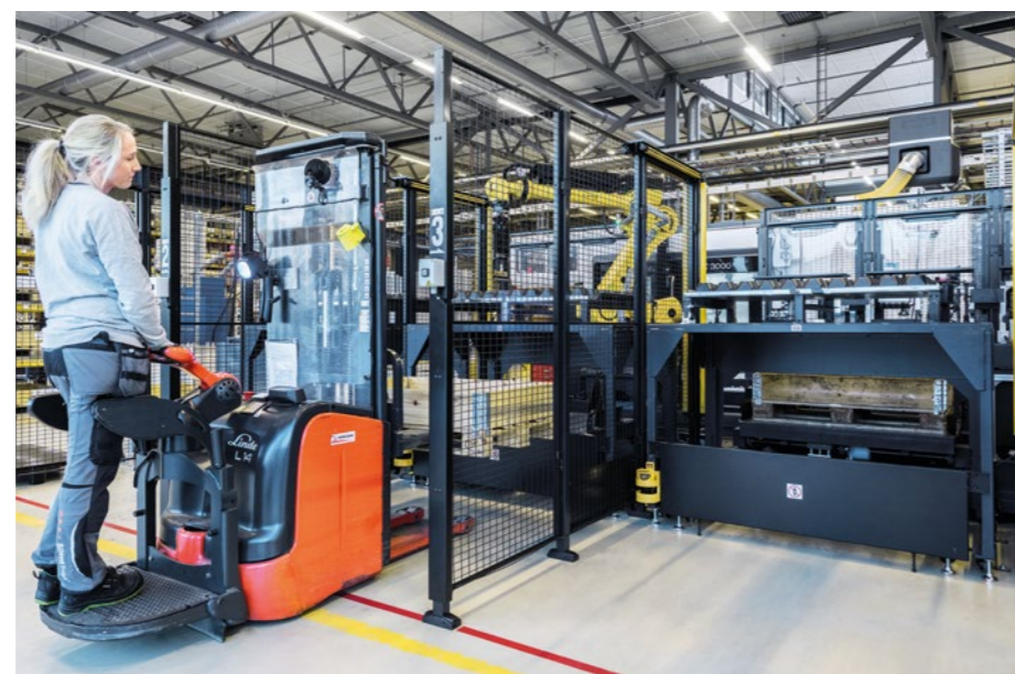
The system has three loading stations, each of which can accommodate a Euro pallet with pre-machined blanks, while the finished parts are deposited at the same time.
