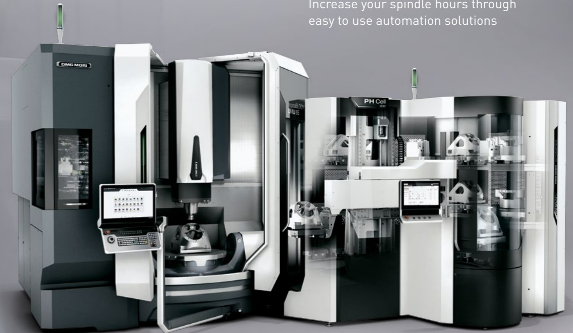
PH Cell 800: Pallet handling with unrestricted access to the working area from the front
