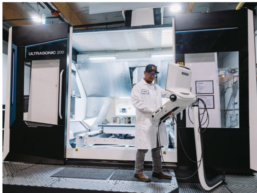
The ULTRASONIC 200 Gantry offers travels of 4,000 x 2,000 x 1,200 mm. The stable foundation of the gantry construction is an optimal basis for the high-precision processing of the mirror segments
