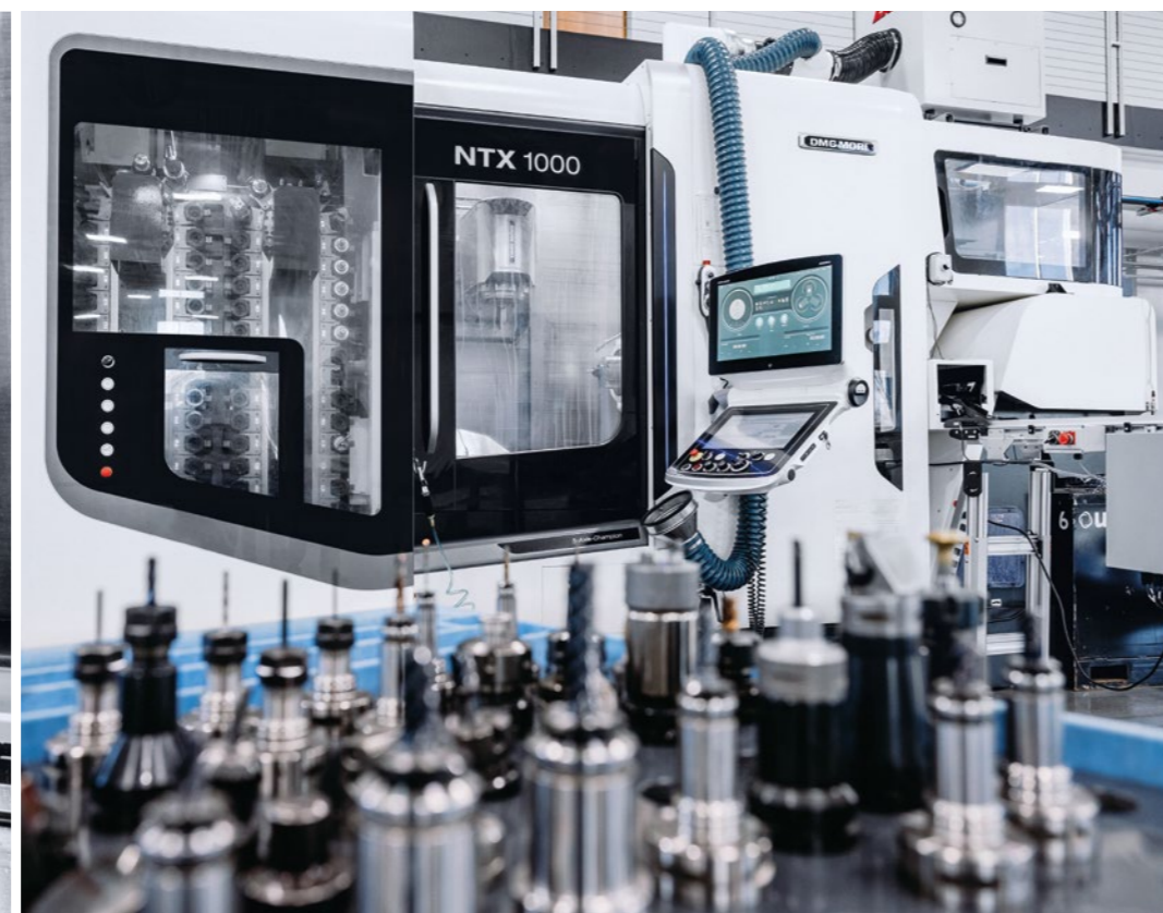
Materials rapidly degrade tools, which may go unnoticed if machinists are not present. Utilizing the tool life management system for lifecycle monitoring and sister tool exchange maximizes unattended process reliability.
