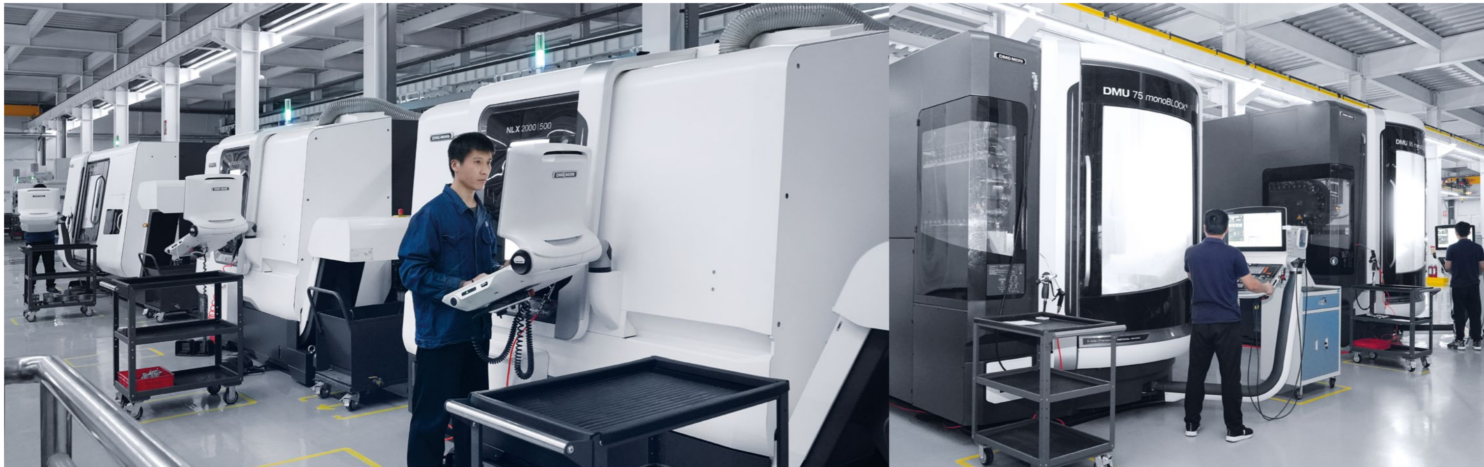
GRANDE-TEK Flow Control Co., Ltd. specializes in the development and manufacture of flow control systems and valves. Two NLX 2000|500 centers and a CTX beta 1250 TC are among the machines used for turning and turn-milling.
